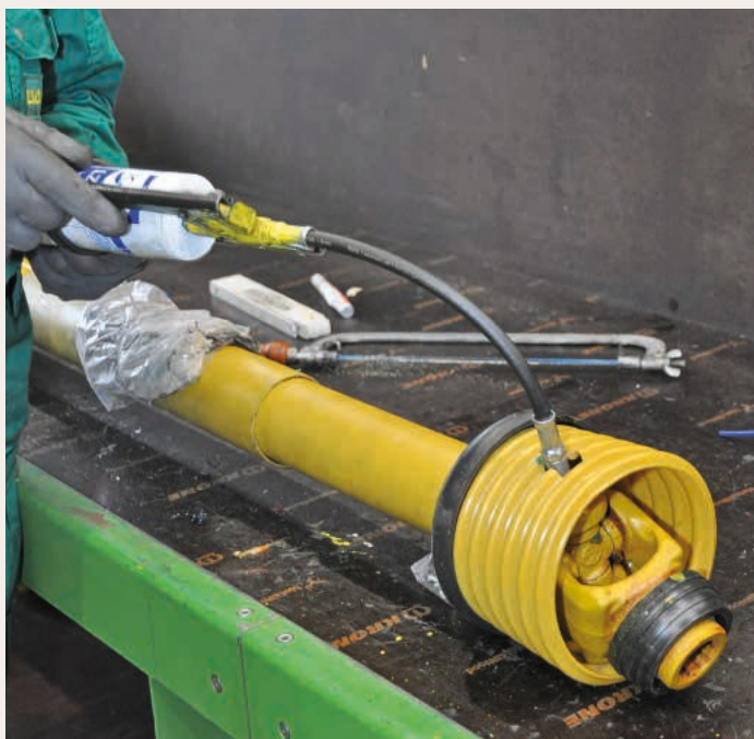
The grease nipples should be filled on both sides of the clevis and at the universal joint.
