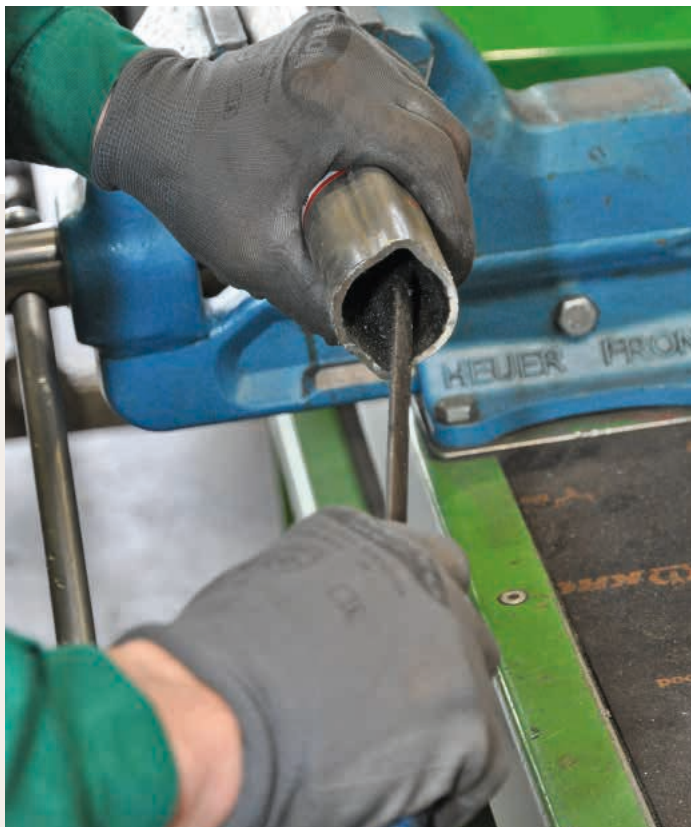
File off rough edges of the flexed pipe – and don't forget a blob of grease inside the profile tube.
