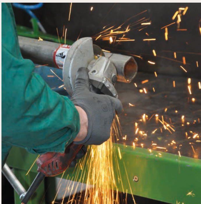
Shortening the pto shaft, the profile tube per flex, and the plastic sleeve using a saw.
