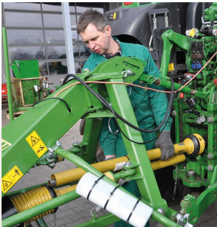
Measure the correct length for the shaft at the mounted implement and mark the length to be shortened.
