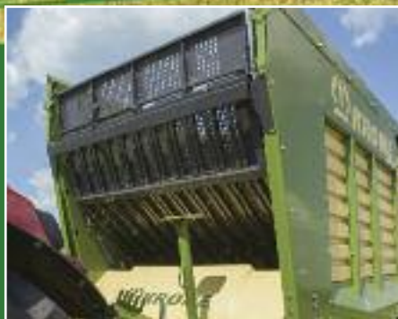
The RX 400 & RX 430 feature a pivoting headboard which swings forwards during loading to increase capacity, then pivots backwards to enhance unloading
