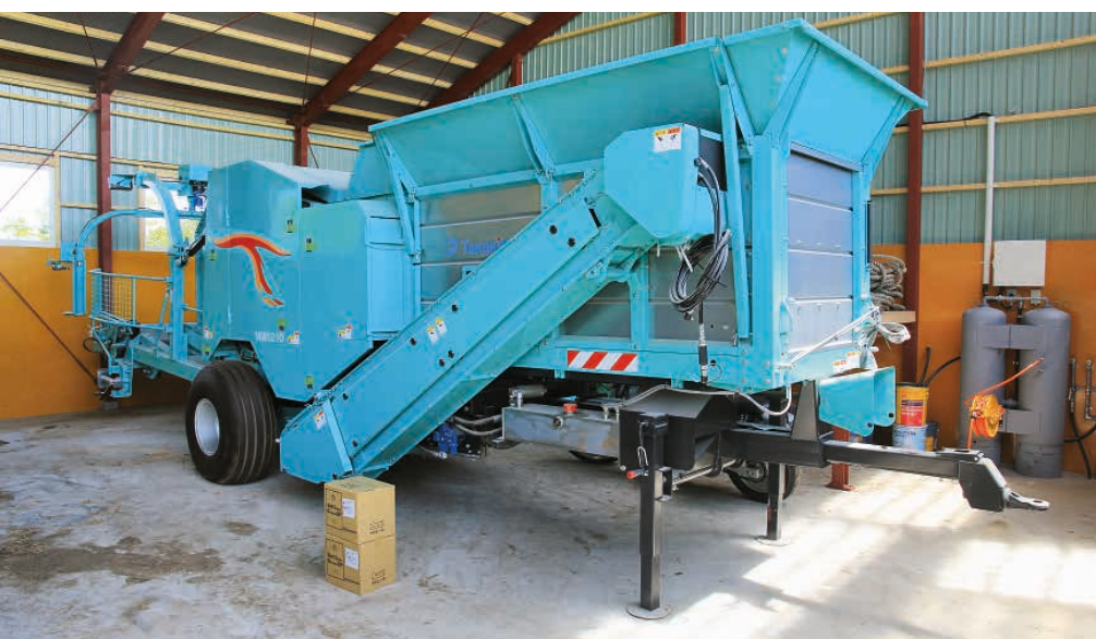
The baler-wrapper combination for maize is built by Takakita and allows silage to be wrapped and deposited directly on farms that have no clamps or silos.
